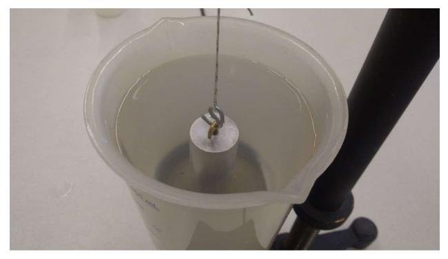
Using the Archimedes' principle, calculate the density ( $\rho$ ) for the measured aluminum cylinder (Equation 3). Compare this result with the known value ( $\rho_{aluminum} = 2700 \text{ kg/m}^3$ ). What is the percent difference?
