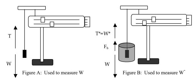
In Figure A, the tension (T) in the string is equal to the weight (W) of the object and is measured by adjusting the two sliding bars until the balance is centered. T = W = mg.
